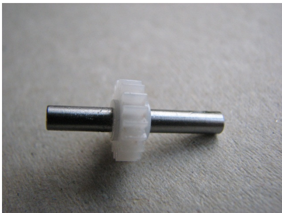
Gear on new axle: note large boss faces chassis centre.
