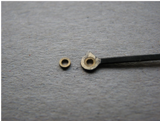
Bush inserted into rod ready for soldering.
