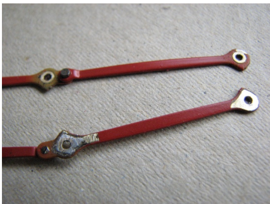
Rods cleaned up after soldering.
